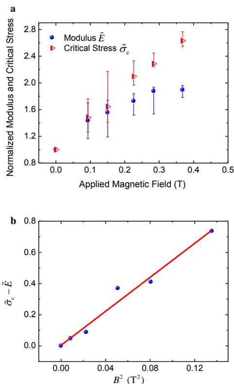
**Fig. 11** (a) Dimensionless Young's modulus and critical buckling stress under different applied magnetic fields. (b) Difference between normalized critical buckling stress and modulus. The filled circles are experimental data, and the line is the linear fit as suggested by the model in Eq. (7).
