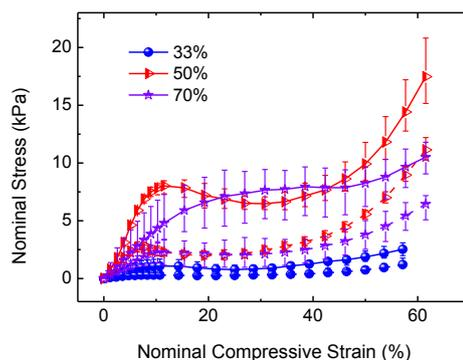
65 **Fig. 9** Measured stress-strain curves of MR-brush samples with different iron particle concentrations. The solid curves show the behavior under a magnetic field of 0.37 T, and the dash curves indicate the zero-field references. The unloading curves are omitted. The error bars show the range of data measured from different portions of the same sample.
