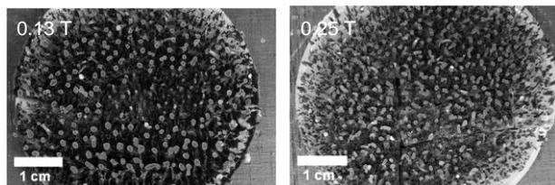
Fig. 6 Top view of the MR-brush samples cured under magnetic field of different strengths as marked.
