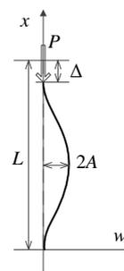
**Fig. 3** Schematic drawing of a single column in the MR-brush structure.
