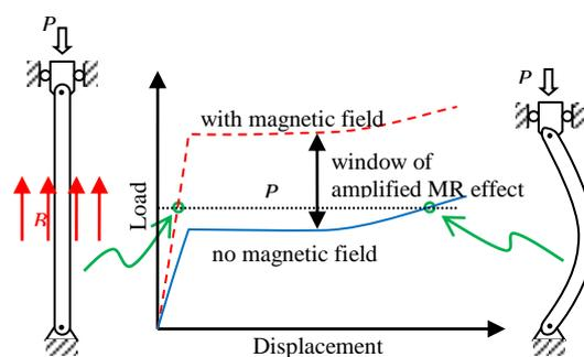
50 **Fig. 1** MR-elastomer column under axial compression. When the load is between the critical value with a magnetic field and that without magnetic field, the responses of the column differ drastically in these two scenarios.
