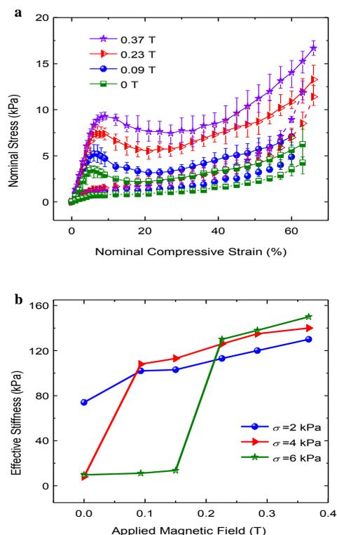
**Fig. 10** (a) Measured stress-strain curves of MR-brush samples with different applied magnetic fields. The solid curves represent the loading cases, and the dash curves indicate the unloading cases. (b) The calculated effective stiffness (nominal stress/nominal strain) during loading at different magnetic fields.
