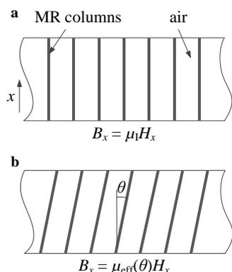
**Fig. 4** Sketch of one horizontal thin slice of the MR-brush structure in the (a) reference state, and (b) buckled state. The magnetic behavior of the column-air system resembles that of a composite material.
