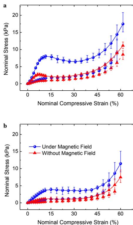
Fig. 7 Measured stress-strain curves of MR-brush samples with different curing magnetic fields at (a) 0.25 T and (b) 0.13 T. Each figure compares the behaviours of a sample under a magnetic field of 0.37 T and without a magnetic field. The solid curves represent the loading cases, and the dash curves indicate the unloading cases. The error bars show the range of data measured from different portions of the same sample.
