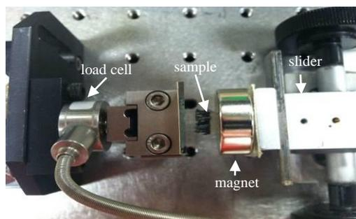
Fig. 5 Experimental setup for measuring the properties of MR brush under magnetic field.
