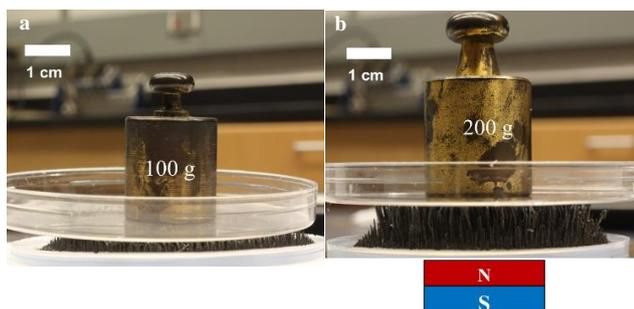
**Fig. 2** Demonstration of the highly tunable stiffness of an MR brush. (a) In the absence of magnetic field, the columns buckled and the structure collapsed with large deformation under a load of 0.1 kgf. (b) Under a magnetic field, the same structure did not buckle and showed little deformation even under a load of 0.2 kgf.
