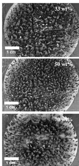
25 **Fig. 8** Top view of the MR-brush structures synthesized with different iron concentrations.
