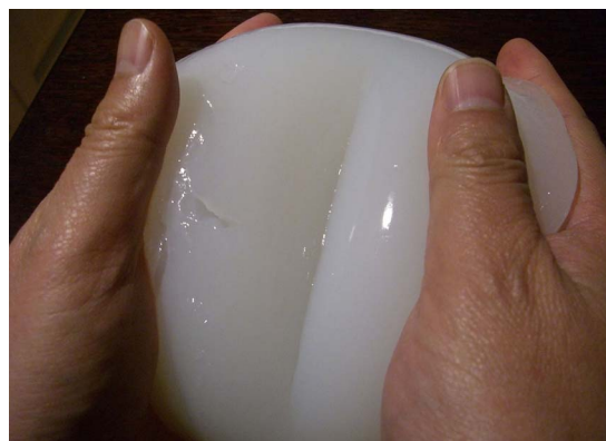
FIG. 1. (Color online) A crease formed on the compressed surface of a popular Chinese food, Liang Fen (a starch gel).
