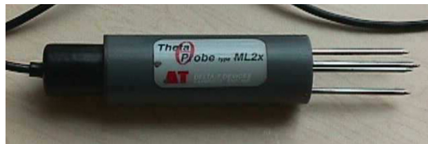
Figure 1. Theta Probe soil moisture sensor. Prongs are 6 cm in length. The volume of soil contributing to the voltage measurement is a cylinder approximately 4 cm wide and 6 cm long.
