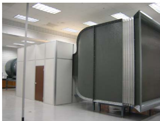
Fig. 1: Low-speed wind tunnel used in the present study
