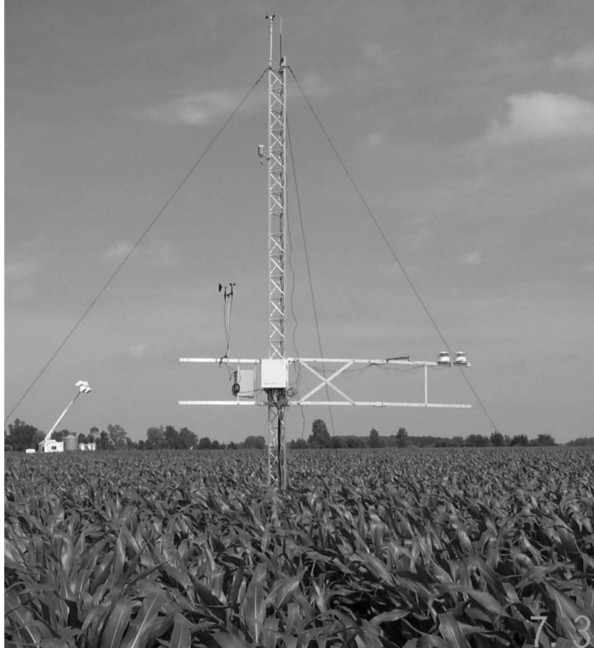
Figure 1: Micro-meteorological tower in Southeastern Michigan, July, 2001. The IRT is on a small arm pointing out of the paper, just to the left of the white pyranometer and pyrgeometer on the end of the long arms.
